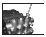
**To Check Valve Assemblies** 1. Loosen plugs (58), take out tension spring (57) and then remove the complete valve assembly (51) with either a valve tool or an M16 hexagon screw.
